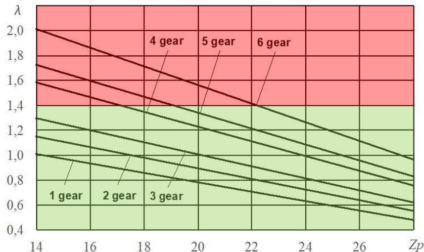
Figure 4 – Dependence of the coefficient of kinematic mode \lambda on the number of teeth of interchangeable drive sprockets Z_o/Z_p
